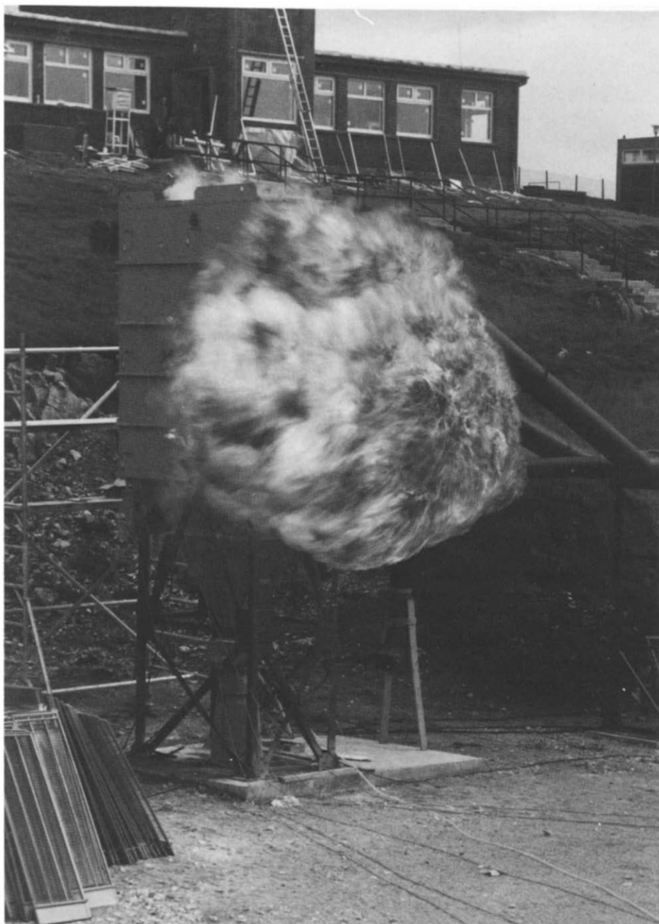
Fig. 5. Rear-vented dust explosion in collector. Phenolic resin powder.
